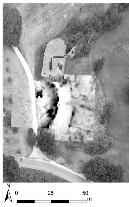
Figure 12.7: Area of the western gate: integration of the orthophoto with images resulting from the 2009 electric resistivity survey and total station survey of some standing structures (by B. Slapšak and R. Plesničar).
