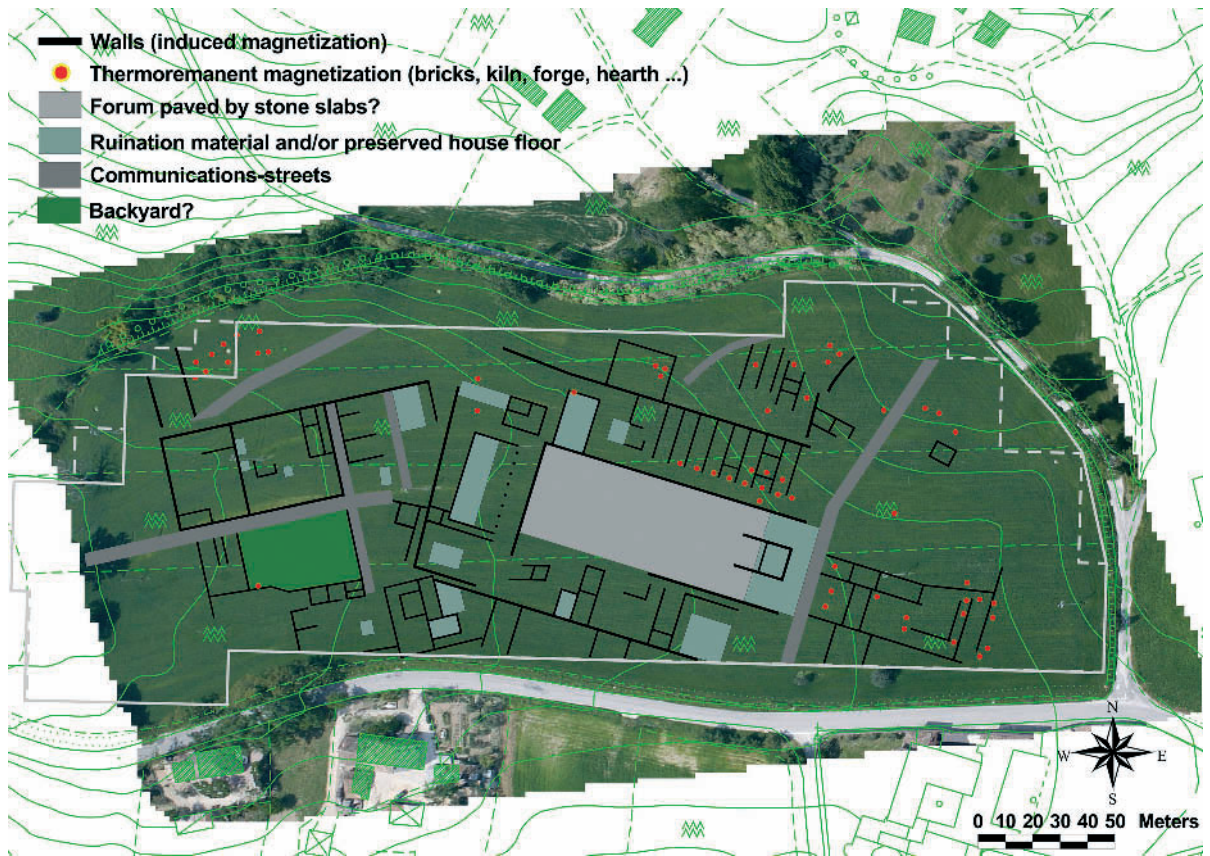
Fig. 23. Interpretation of geophysical results of the Trea survey, presented on the topographic map and a rectified oblique aerial photograph.
