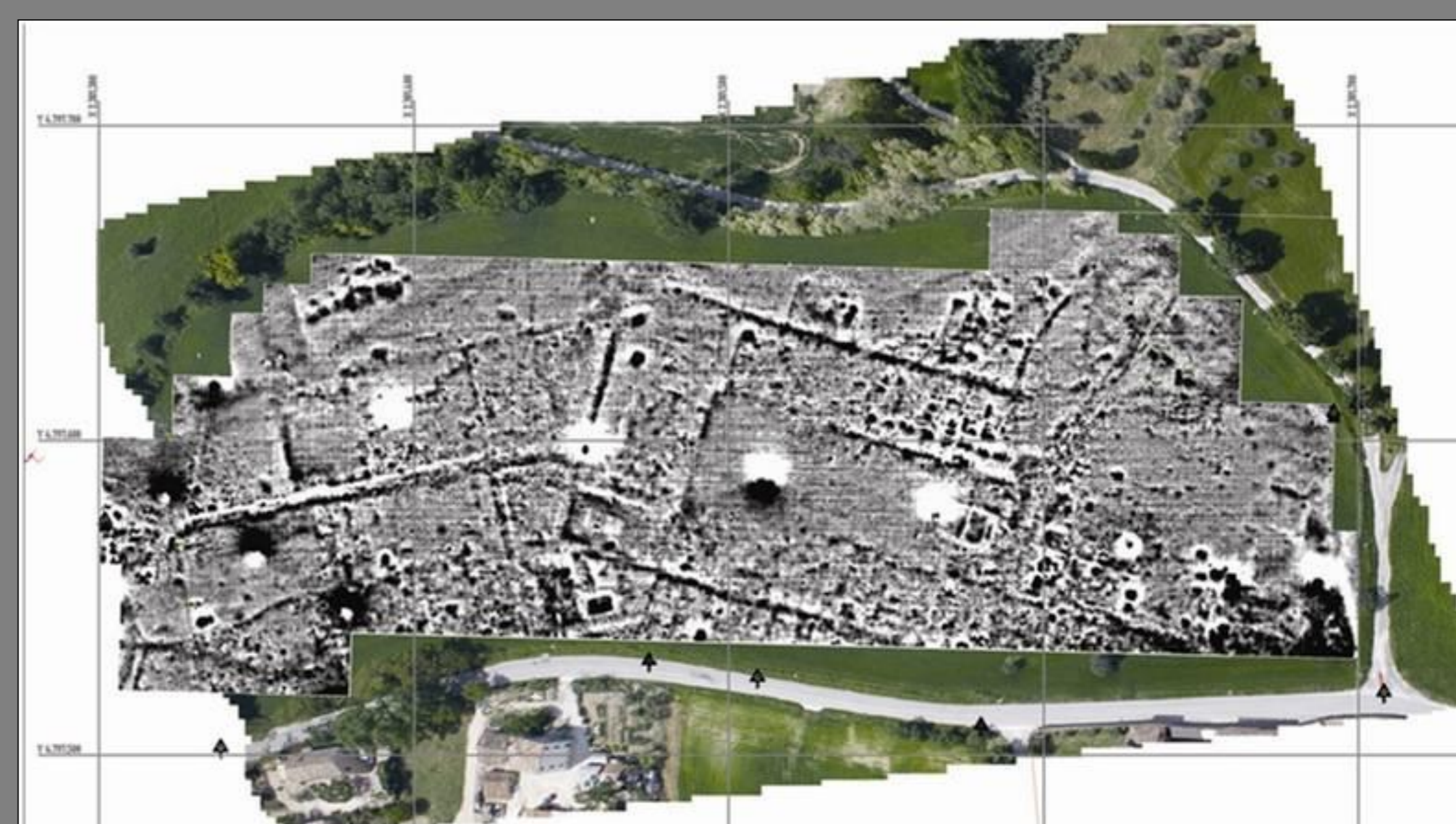
Central area of Trea (results of the magnetic survey Geometric G-858 ).
