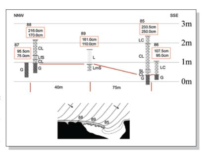
**Figure 14** The hypothesis of a spit south of Potentia, illustrated with hand augerings (location see figure 10) and a textbook example (white = sea; black = land; speckled = spit), on which the locations of the augerings are added. Textbook example: Pannekoek & Van Straaten (1992).
