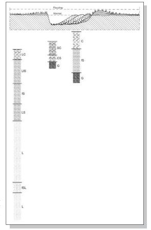
**Figure 8** Augerings 8, 9 and 10, cross-sectioning through palaeochannel I, linked with a school-book example of a meander bend (translated from Pannekoek & Van Straaten, 1992).
