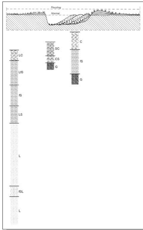
**Figure 8** Augerings 8, 9 and 10, cross-sectioning through palaeochannel I, linked with a school-book example of a meander bend (translated from Pannekoek & Van Straaten, 1992).
