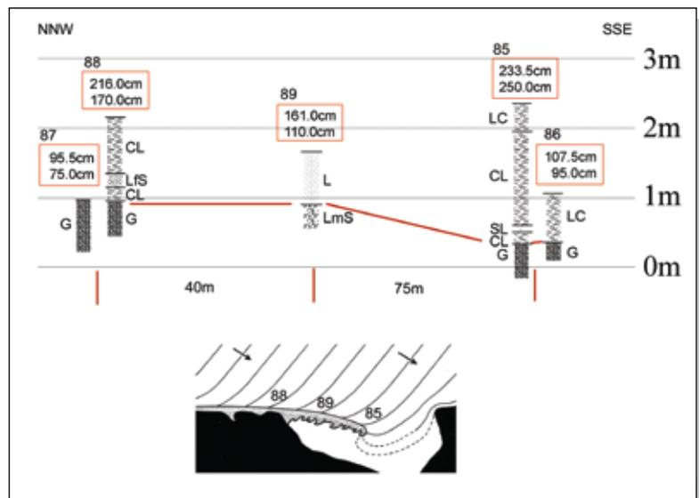
**Figure 14** The hypothesis of a spit south of Potenza, illustrated with hand augerings (location see figure 10) and a textbook example (white = sea; black = land; speckled = spit), on which the locations of the augerings are added. Textbook example: Pannekoek & Van Straaten (1992).
