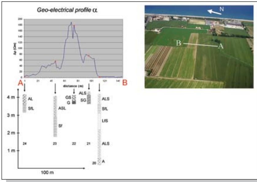
**Figure 7** Geo-electrical transect  $\alpha$ , type-section through palaeochannel I.
